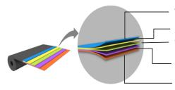
TREATED MODIFIED PRINTABLE SURFACE MODIFIED INTERMEDIATE LAYER WHITE CAVITATED MODIFIED OPP CORE **MODIFIED INTERMEDIATE LAYER**
